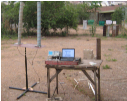
Fig. 3: The open-area experimental setup for the proposed helical antenna array
