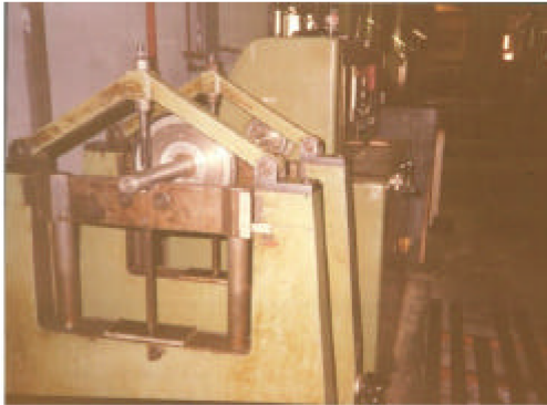
Plate 1: The flywheel mounted on balance machine
