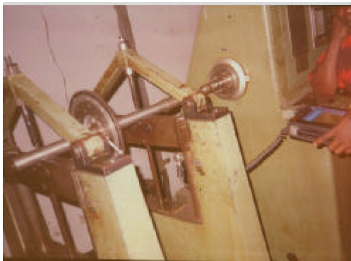
Plate 2: Taking vibration and balance data
