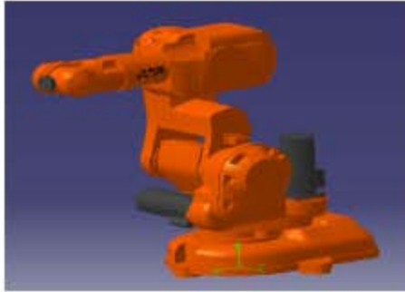
Fig. 5: ABB IRB 140. IRB 140, Axis: 6, Reach: 810 mm, Payload: 5 kg Repeatability: 0.03 mm
