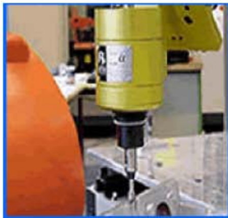
Fig. 1: Tool in hand configuration
