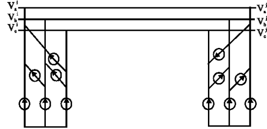
Fig. 5: Representation of the flow of currents due shunt capacitances
