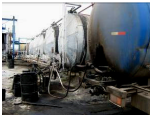
Fig. 7: A view of pipes connections used to supply heat to flowing bitumen (Courtesy: Julius Berger Nig. Ltd.)
