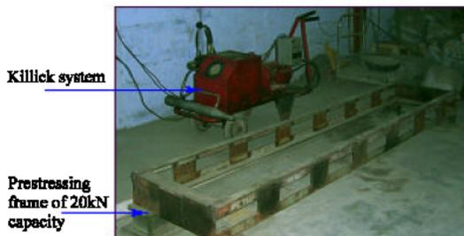
Fig. 2: Killick system of prestressing and prestressing steel frame
