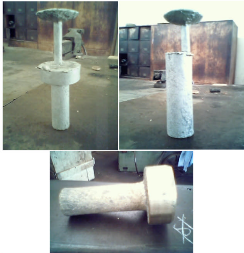
Fig. 4: Plates of the products after casting before machining
