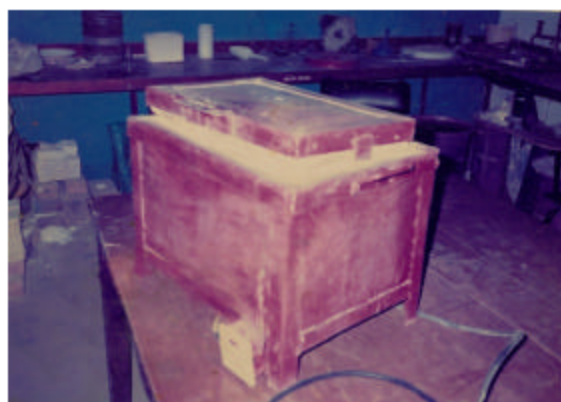
Fig. 2: Showing a top-loading electric oven constructed with insulating bricks made from sawdust and kaolin mixture
