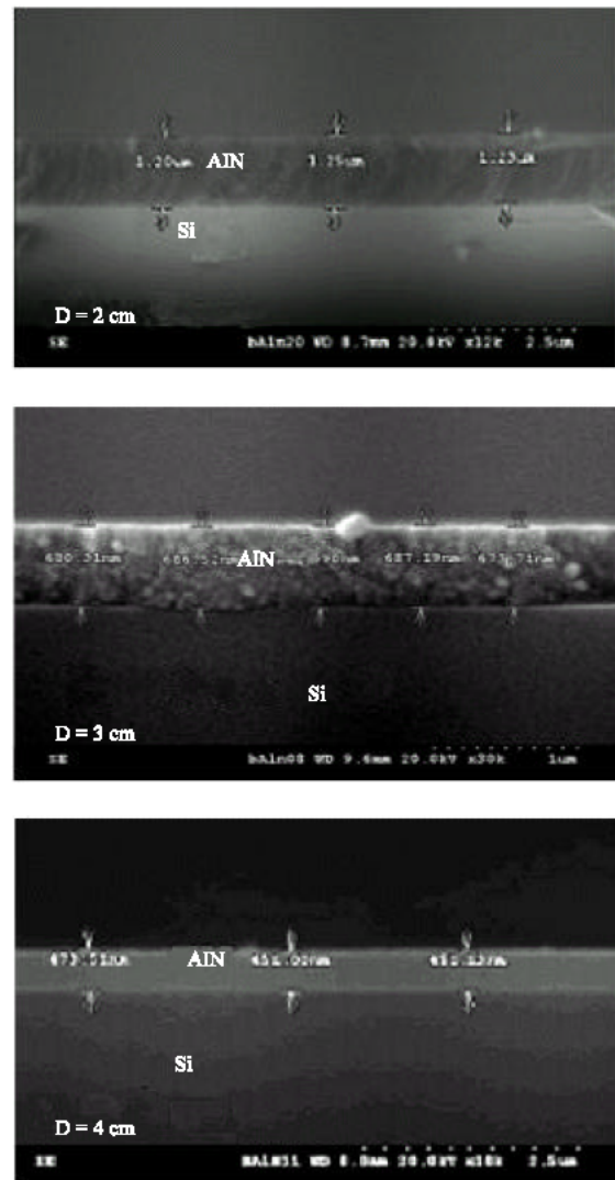
Fig. 7: SEM cross section images at different Substrate Target distances
