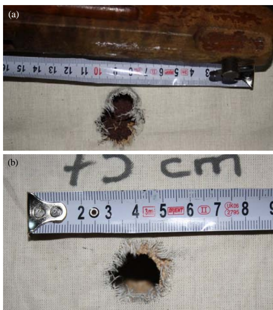
Fig. 5: a) The defect on a cotton target by shot of the modified shotgun: the range of fire is 75 cm; b) the defect on a cotton target by shot of the non-modified shotgun: the range of fire is 75 cm
