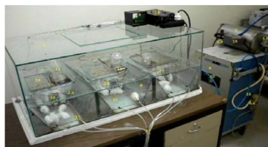
Fig. 1: Appearance of DE Model; 1: DEC (Dry Eye Cabinet); 2 (a-c): EAD (Experimental Animal Division); 3: The subjects; 4: AC (Air compressor); 5: AC tube; 6 (a-c): Water separator; 7: Flowmeter; 8: Desiccators' containers; 9: Control board; 10: Fan; 11: Humidity-Temperature monitor; 12: Mobile glass plates; 13: Watering; 14: Feeder; 15: Air inlet holes; 16: Pneumatic pipes; 17: Flexible inhalation hose; 18: Fan switch board; 19: AC pressure monitor; 20: AC pressure gauge
