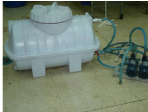
Fig. 1: A photograph showing the 250 L capacity storing tank with attached 2 pumps
