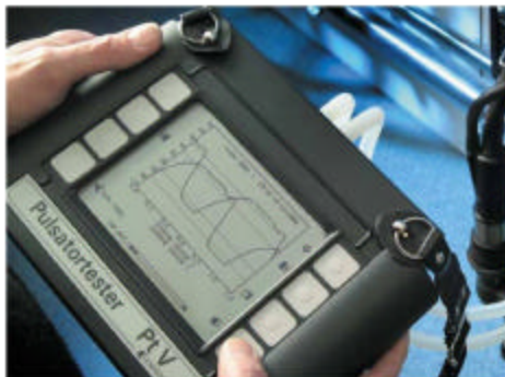
Fig 1: Electronic vacuum recorder and pulsation analyzer
