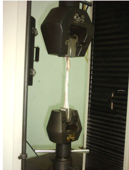
Fig. 1: Servohydraulic mechanical test system. The tendon-graft tendon unit is under the test
