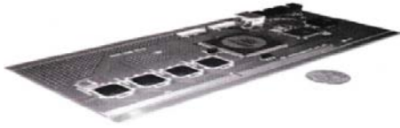
Fig. 5: The 40-ch WSFE board made with prototype WSFE ASICs. The board consists of four bare chips, a FPGA (Altera Flex) and USB controller, etc.
