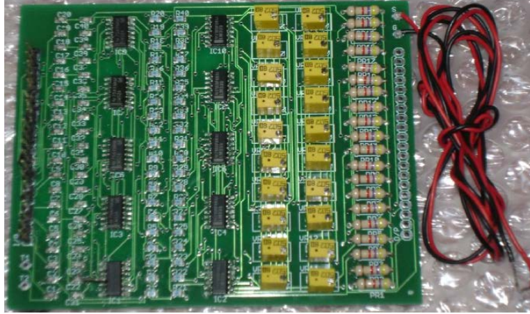
Fig. 2: The board of the proposed module created by EAGLE
