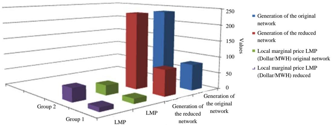
Fig. 4: Comparison of generation amounts and LMPs of the original network and the reduced network regarding the congestion line 8-2
