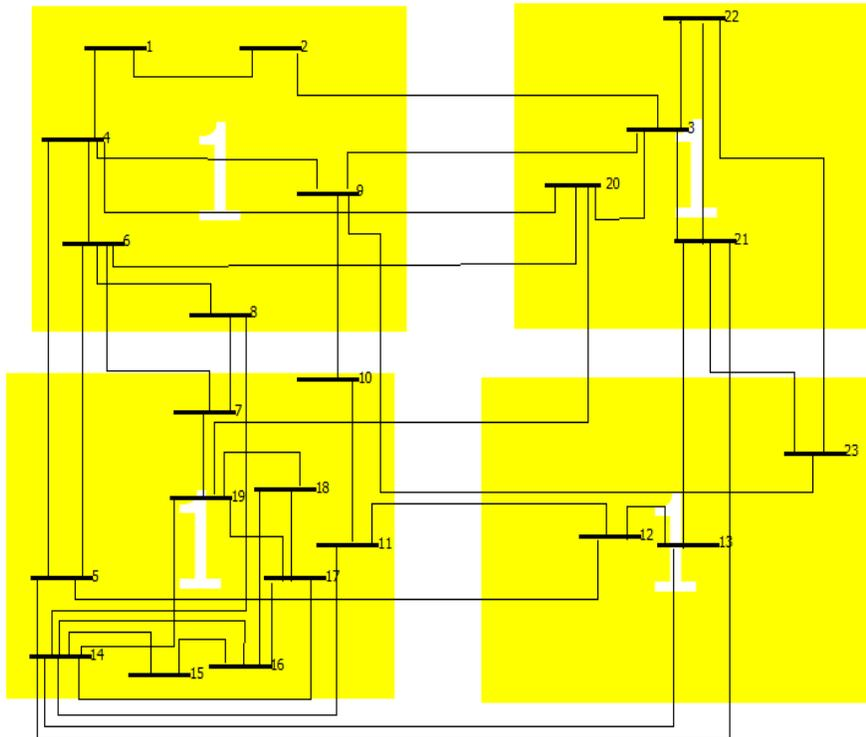
Fig. 6: Reduction of IEEE 118-busbar system based on bus bar arrangement in Table 3
