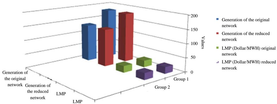
Fig. 3: Comparison of generation amounts and LMPs of the original network and the reduced network regardless of the congestion line
