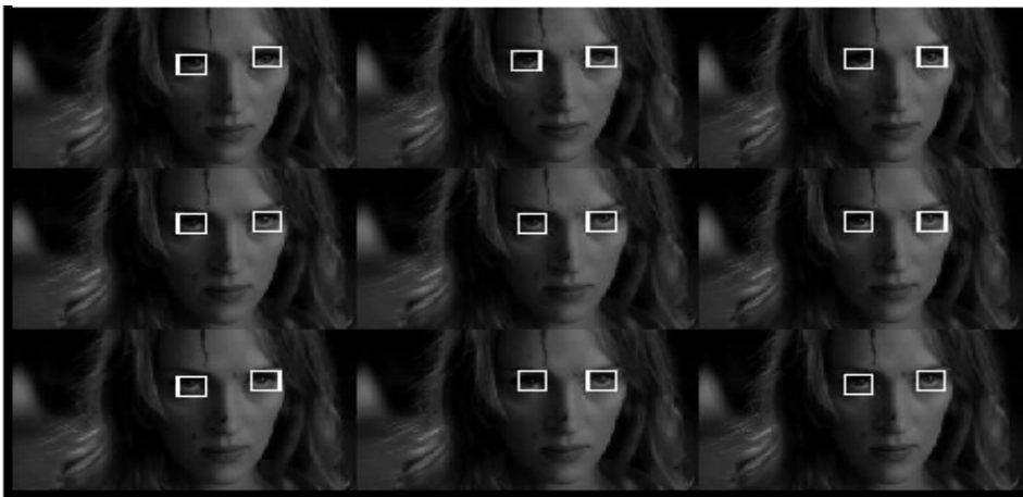
Fig. 10: An example of eye tracking using fixed templet matching for nine frame
