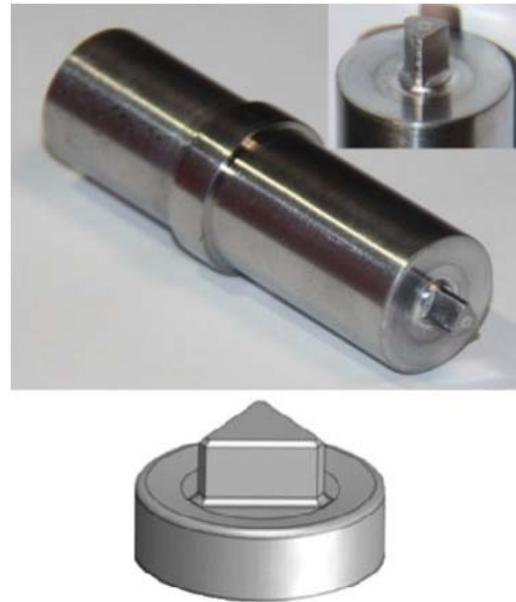
Fig. 2: Schematic and Image of beveled triangle-shaped pin
