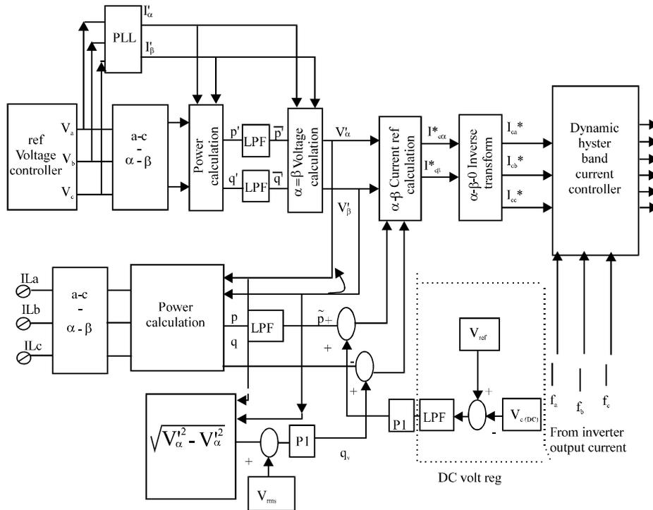
Fig. 4: Control system of shunt converter in UPLM
