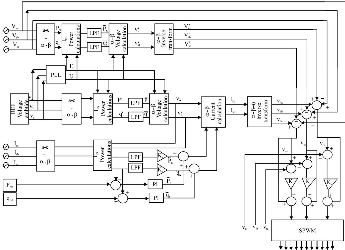
Fig. 5: Control system of series converter in UPLM
