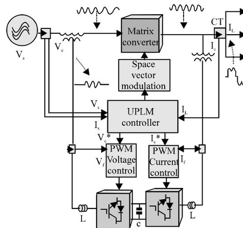
Fig. 1: Basic configuration of universal power line manager
