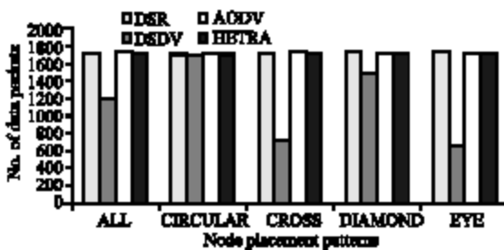
Fig. 14: Number data packets delivered in WSN with various routing algorithms and TCP/Exp congestion control
