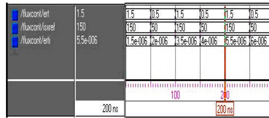
Fig. 3: Result of flux controller. Input: Error values of i_{mref} and i_{mr} . Output: Reference value of current in X-axis ( i_{xrefref} ) using PI action
