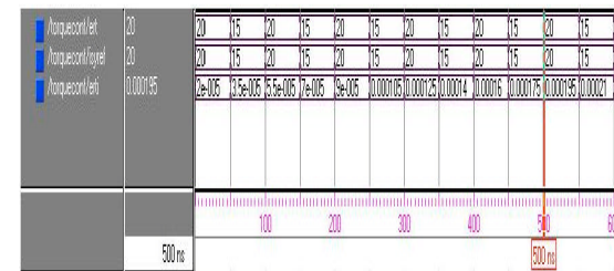
Fig. 5: Result of Torque controller. Input: Error values of T_{refref} (from Speed Controller) and T_e (from flux Model) Output: Reference Value of current in Y-axis ( i_{yrefref} ) using PI action
