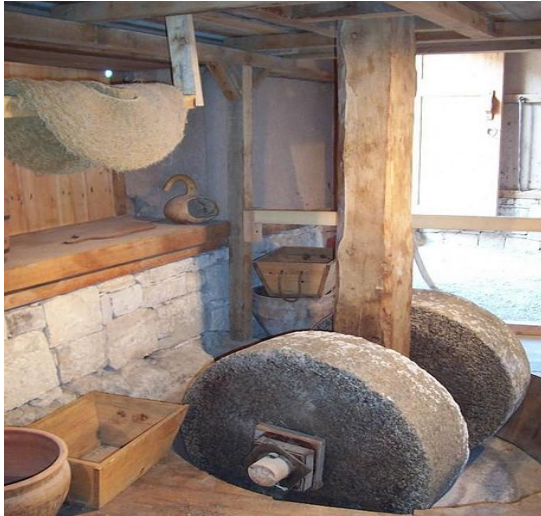
Fig. 3: Old olive oil extraction machine (oil-press)
