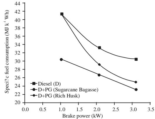
Fig. 4: Specific fuel consumption vs. brake power
