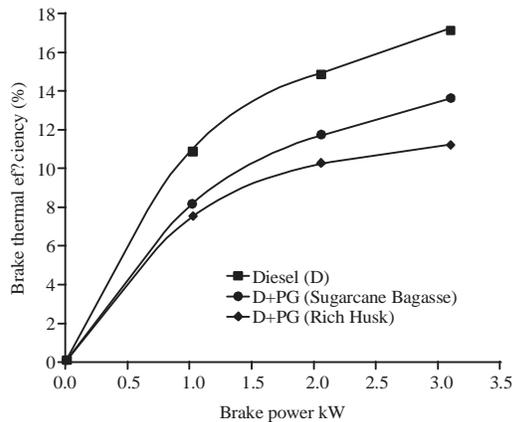
Fig. 3: Brake thermal efficiency Vs. Brake power
