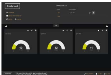
Fig. 10: Customized GUI using freeboard to display Max. current delivered by transformer
