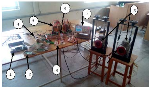
Fig. 8: Hardware setup; 1. FPGA 2; Sensor 3; Power supply 4; Rectifier 5; Isolation transformer 6; Inverter Units 7; DSO 8; Induction motors
