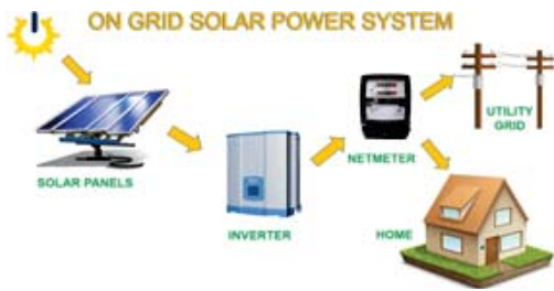
Fig. (3-4): Flow power in grid on solar system
