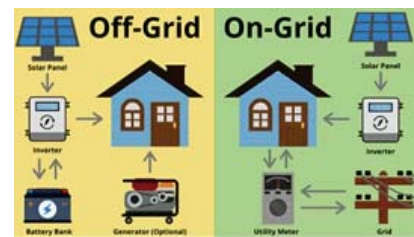
Fig. (3-2): Grid off/on solar system
